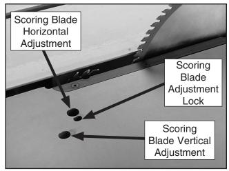
Figure 35. Scoring blade adjustment controls.
